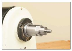
Thread the bottle stopper chuck onto your lathe headstock.
