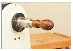
Once pre-shaped, loosen the tailstock hand wheel and remove the live center from your project. Move the tailstock out of the way. Decide what your profile is going to be and turn your blank. Your final diameter at the base of the blank should match your chuck collar diameter. Sand through 320 grit, finish and polish your project to your liking. Remove your project from the lathe and chuck.
