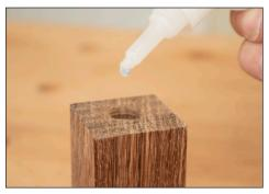
Apply thin viscosity C/A glue on to the threads of the hole. Be sure to evenly cover the threads. This helps to reinforce the threads to prevent stripping. Let the glue dry overnight so that it is 100% dry and 100% cured.
