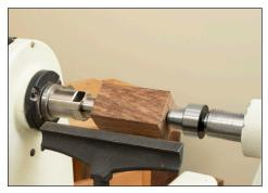
Once the glue is completely dry, thread the blank back on to the chuck. Install a live center on to the tailstock and secure the floating end of the blank as shown above.
