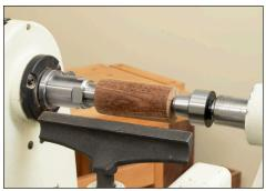
Pre-shape your blank as much possible with the tailstock in place to prevent excess stress on the blank.
