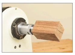
Thread the drilled bottle stopper blank onto the threaded stud end of the bottle stopper chuck. Since the hole on the blank is smaller than the threaded stud size, it is important to thread the blank onto the chuck slowly. As you thread the blank on to the chuck, be sure to keep steady even pressure on the blank. This will help the threads cut into the wood and help produce a threaded hole in the blank.
