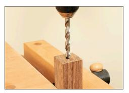
Drill a hole on your center mark. The hole should be approx. <sup>3</sup>/<sub>4</sub>" deep. In our example we are using an 11/32" drill bit since our chuck thread size is 3/8".
